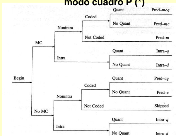
Figure 10.21 The macroblock type decision procedure in P pictures. m : motion compensated, c : at least one block coded, q : quantizer changed, d : default quantizer used, pred : predictive (forward) mode, MC : motion compensation mode.
