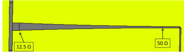
Figure 4.12: Taper structure in the MIMO system
