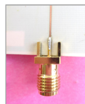
Figure 8.2: SMA connected at the end of the microstrip line port
