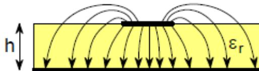
Figure 2-23: Field lines in microstrip patch
