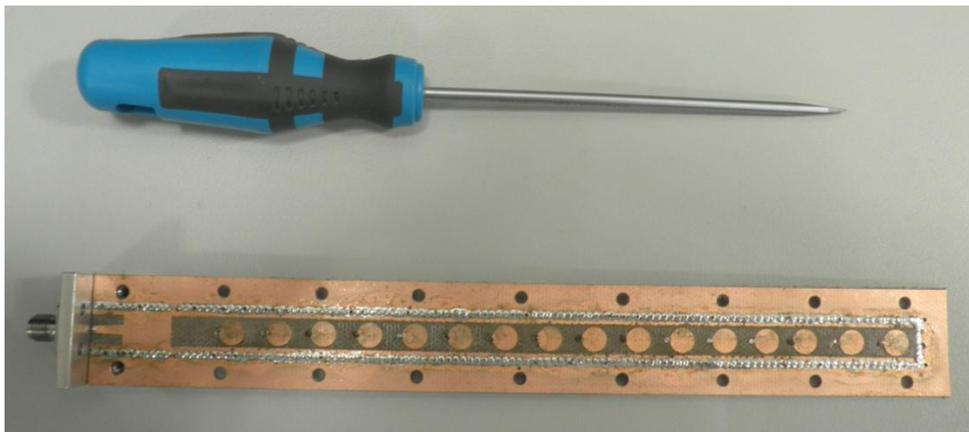
Figure 5-11: Mounted and soldered connector in the SIW
