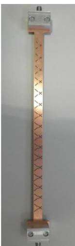
Figure 2-31: Linear slotted array antenna
