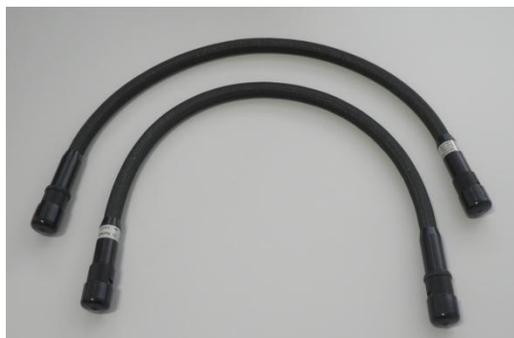
Figure D-2: Coaxial cables used for measurements with VNA, property of EPS
