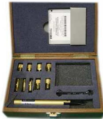
**Figure D-3: Content of the calibration kit 85052D de Agilent Technologies, property of EPS**
