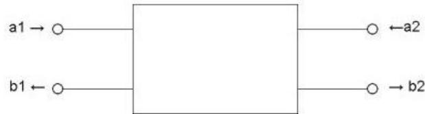
**Figure 2-11: Two-port circuit with incoming and outgoing power waves**
