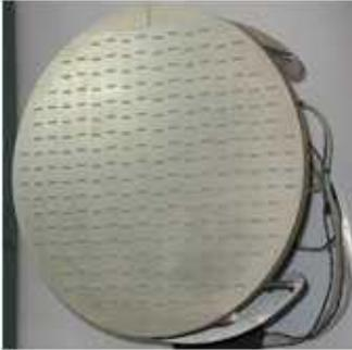
Figure 2-6 Circular slot antenna for satellite communications in band Ku
