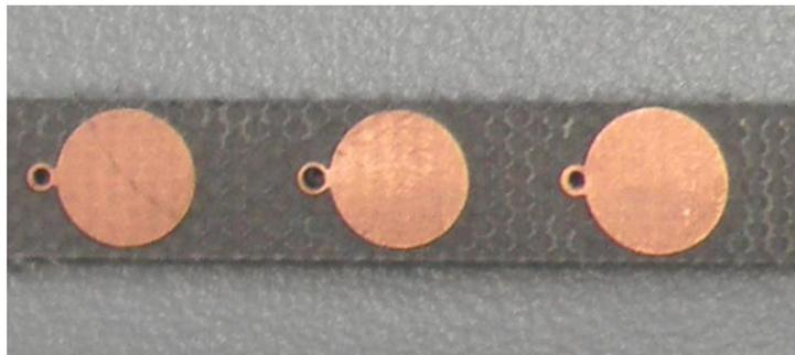
Figure 5-5: Detailed view of the lower patches of the 14<sup>th</sup>, 15<sup>th</sup> and 16<sup>th</sup> elements (from left to right), which include the three different patch structures designed
