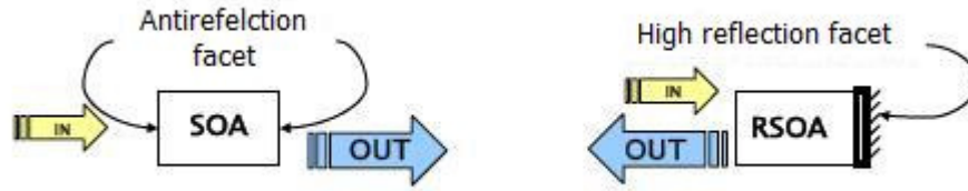
Fig. 3-9: SOA and RSOA transmission diagram
