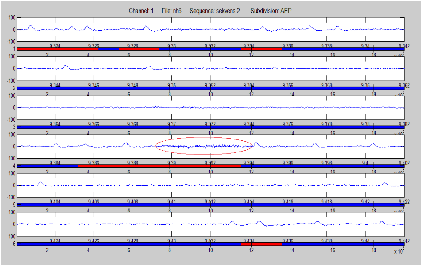
Figure 18: One minute of EEG signal after the ocular and the muscle filter is represented (10 seconds each row). Below the signal we can see a colour bar. Blue means it is useful data, and red means it has been removed by the ocular filter. The red circle marks a muscle artefact that has been removed.
