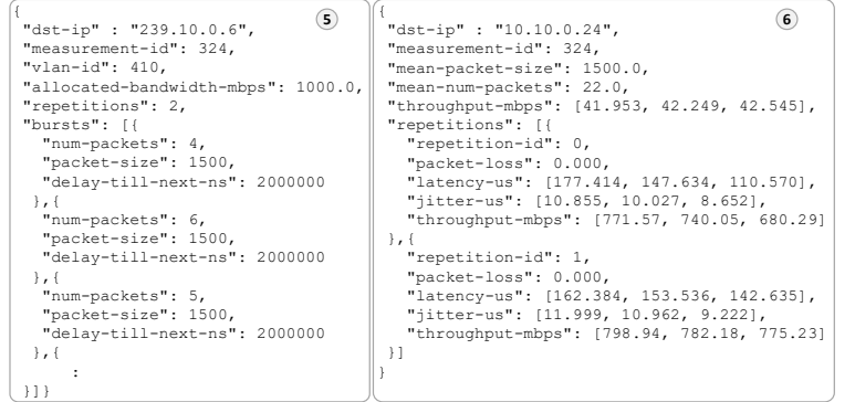
Fig. 8. JSON messages for measurement configuration and results.
