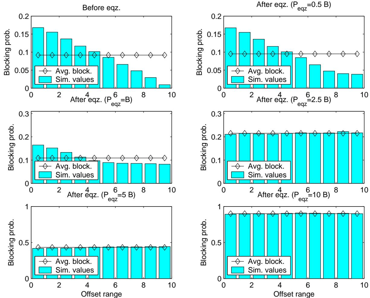
Fig. 8. Blocking probabilities before and after equalisation with different targeted blocking probabilities: Before equalisation (top-left); After equalisation with  $B_{eqz} = 0.5B$  (top-right); After equalisation with  $B_{eqz} = 1B$  (middle-left); After equalisation with  $B_{eqz} = 2.5B$  (middle-right); After equalisation with  $B_{eqz} = 5B$  (bottom-left); and, After equalisation with  $B_{eqz} = 10B$  (bottom-right).
