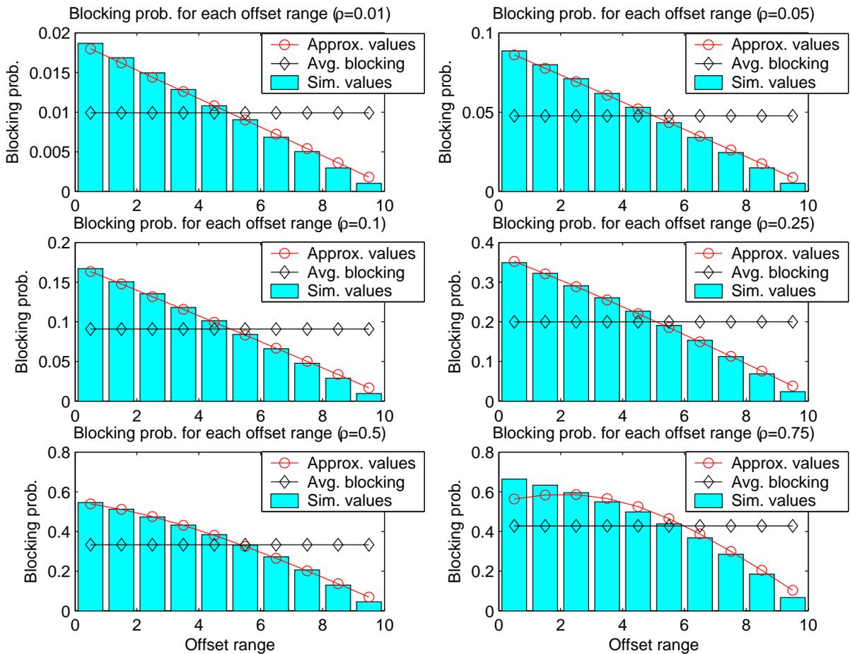
Fig. 7. Blocking probability observed by each offset range in several conditions:  $\rho = 0.01$  (top-left),  $\rho = 0.05$  (top-right),  $\rho = 0.1$  (middle-left),  $\rho = 0.25$  (middle-right),  $\rho = 0.5$  (bottom-left), and  $\rho = 0.75$  (bottom-right)
