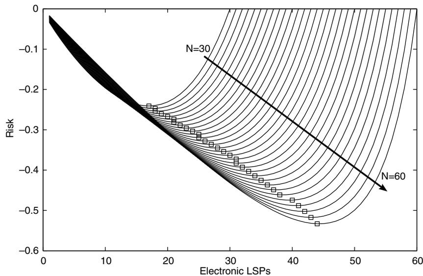
Fig. 11. Risk versus optimal number of electronic LSPs for a total number of LSPs in the range 30–60.
