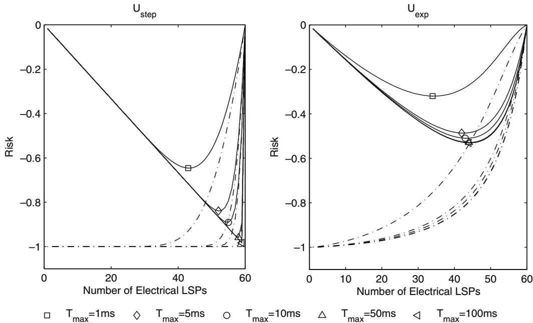
Fig. 3. Bayes risk curves and optimal decisions (minimum values of risk) for several  $T_{max}$  values assuming hard real-time utility (left) and elastic utility (right) functions. Dashed line = Utility.
