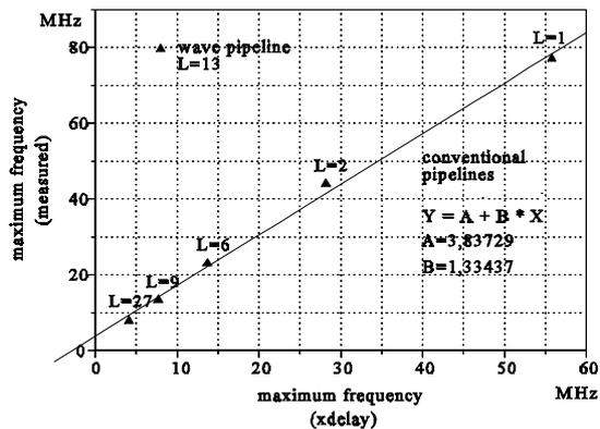
Fig.5: Simulated vs. measured frequency operation. Conventional and wave pipelines (L=logic depth in LUTs)
