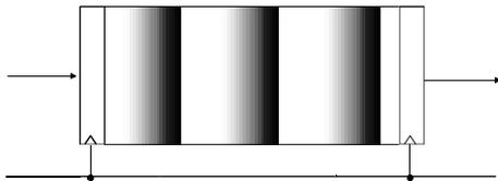
Fig.1c: For this frequency, the wave that enters in  $t=kT$  reaches the reception register after  $(k+2)T$ , but it is stable before the clock edge  $(k+3)T$ . Once again, each result is latched properly.
