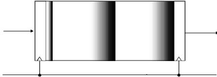
Fig.1b. A frequency increment produces a setup window violation in the reception register bank.
