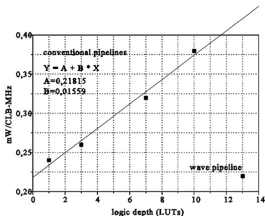
Fig.6: mW per CLB-MHz figure vs. logic depth. Conventional and wave pipelines.
