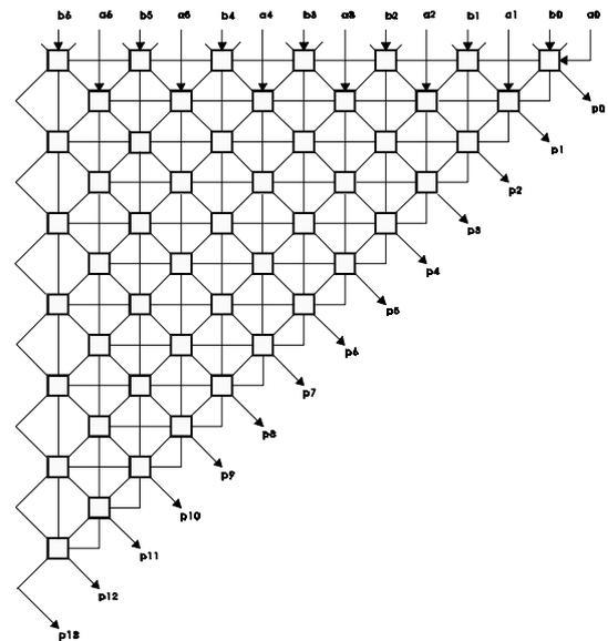
Fig.2: 7-bit Guild array multiplier.
