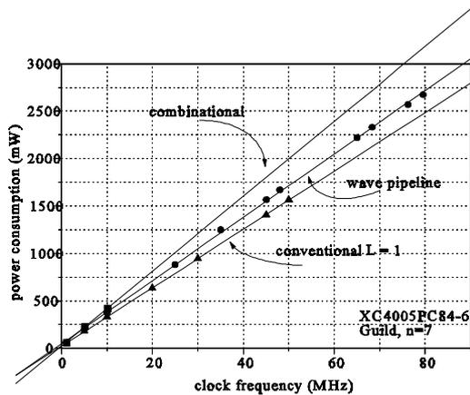
Fig.7 :Power consumption vs. frequency. Conventional and wave pipelines
