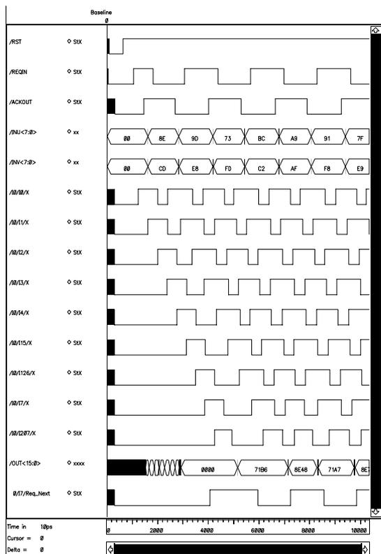
Fig. 1: The signals named with X, control the latches of successive stages ( the latches are transparent when “0” and locked when “1”). In this case, the frequency is close to maximum pipeline speed ; thus, the usual behaviour of a non-overlapped two-phase pipeline can be observed.
