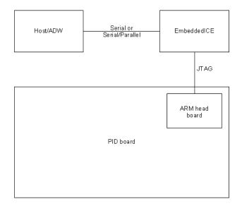
Figure 3-1 A typical debugging set-up
