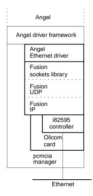
Figure 13-14 Angel, Fusion ,and PID hardware
