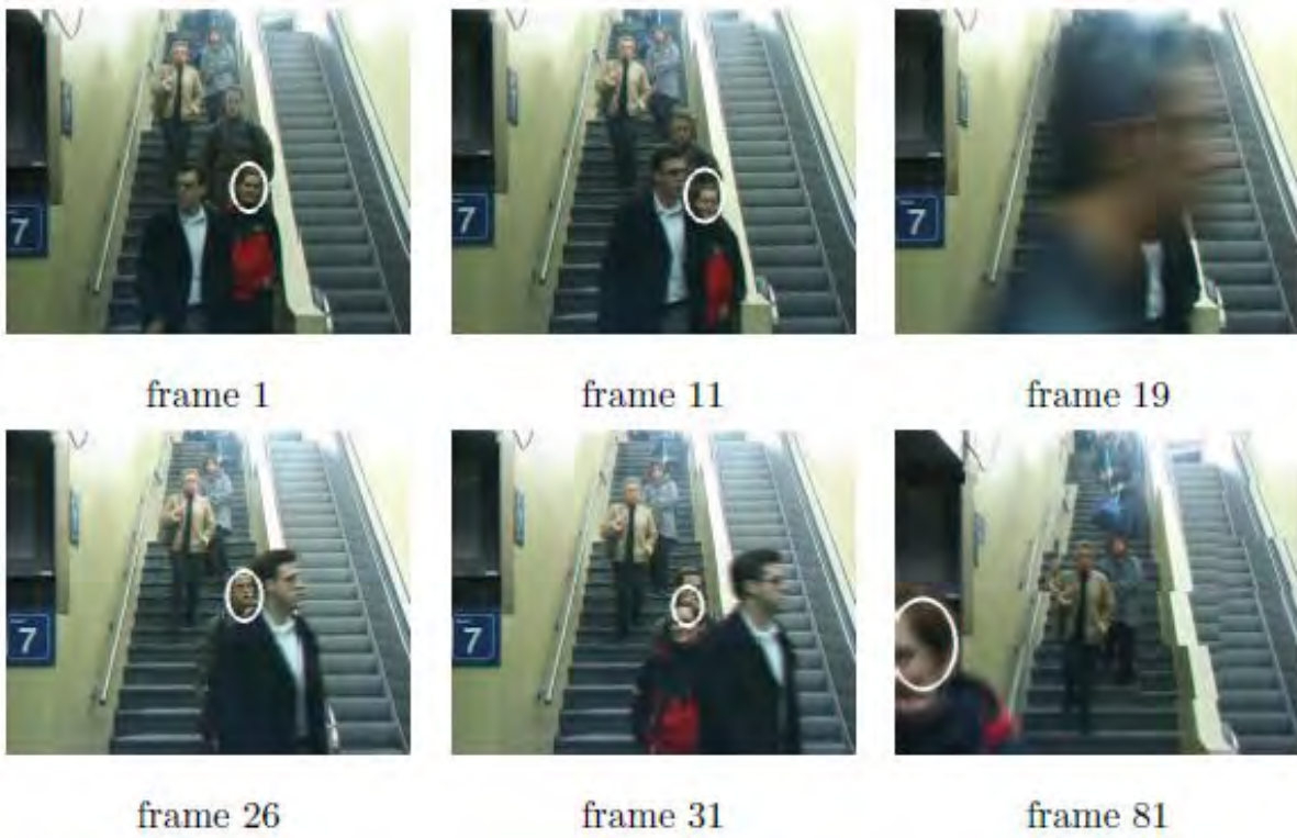
Figure 3.12: Example of the color-based particle filter algorithm for a sequence with occlusions (frame 19) and scale changes (frames 31 and 81) [50]
