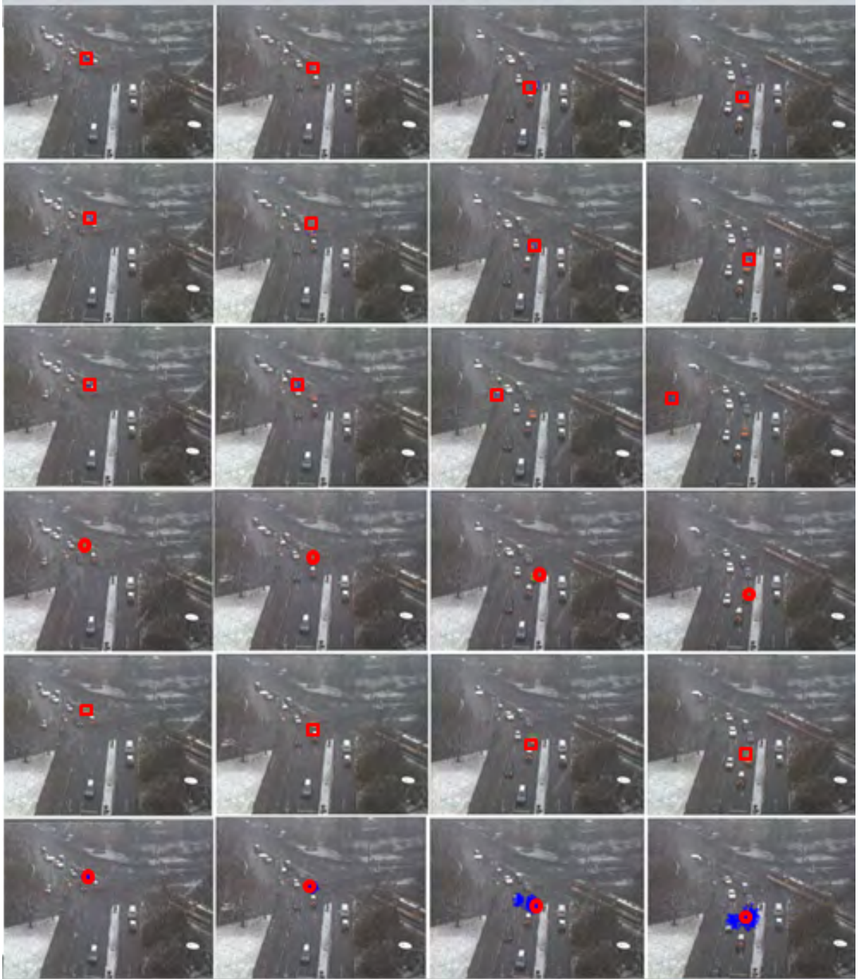
Figure 5.14: Example of noise with a Level 3 sequence. Frames: 1, 50, 100, 150. Algorithms (from top to bottom rows): CBWH, MS, MSA, SOAMST, TM, PF.
