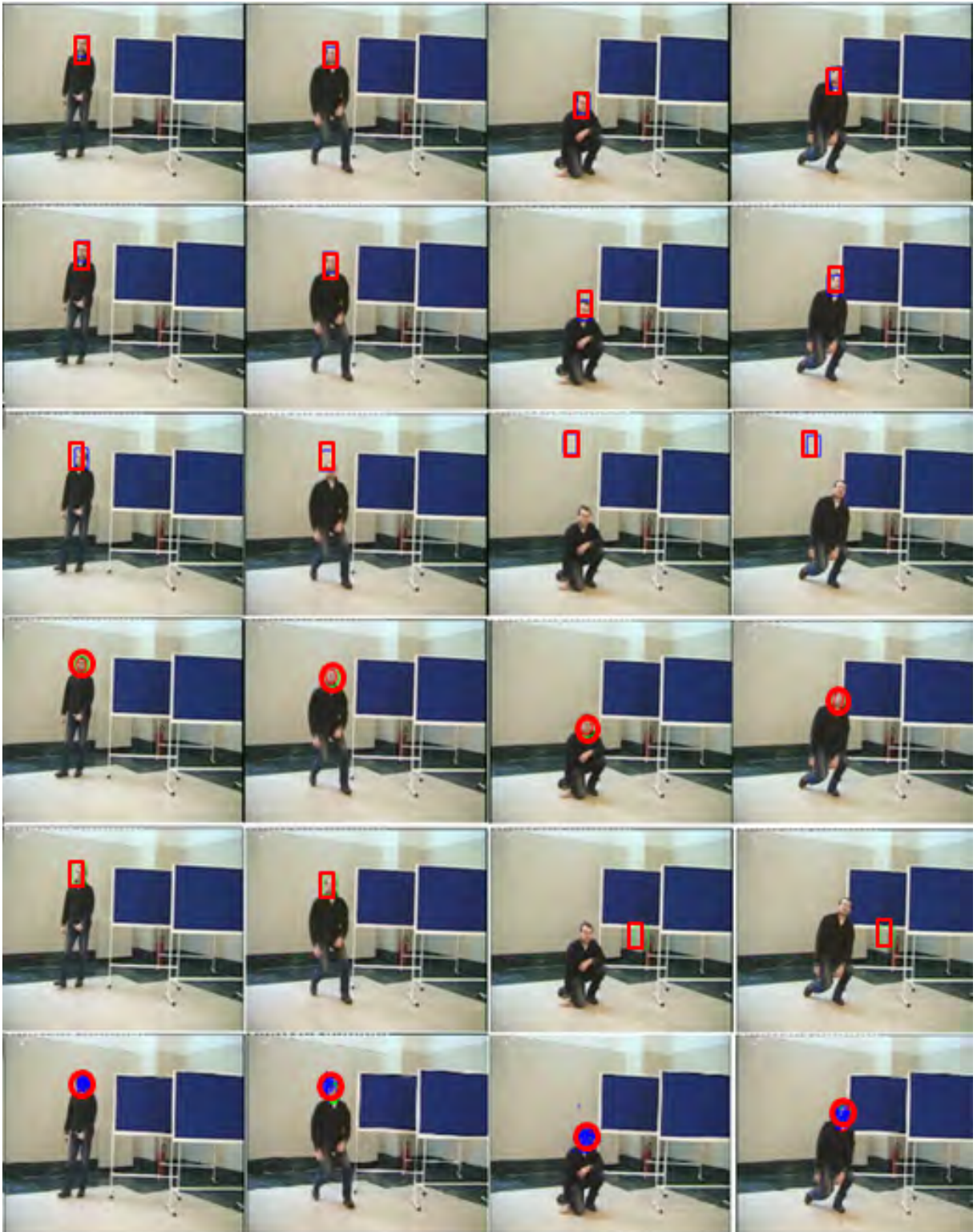
Figure 5.8: Example of complex movement with a Level 3 sequence. Frames: 1, 20, 40, 60. Algorithms (from top to bottom rows): CBWH, MS, MSA, SOAMST, TM, PF.
