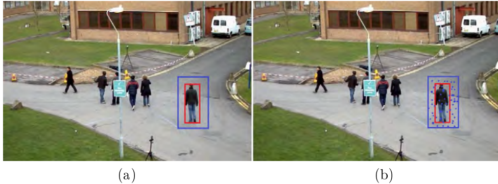
Figure 2.4: Prediction of motion approaches: (a) Exhaustive search, (b) Selective search (where blue points represent the selection)
