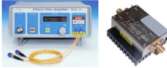
Figure 8.4: Optical amplifier, EDFA (left) and RF amplifier (right).
