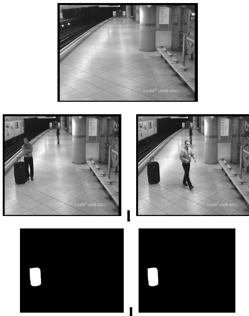
Figure-52: Background image, two frames and two foreground object masks of the abandoned object dataset
