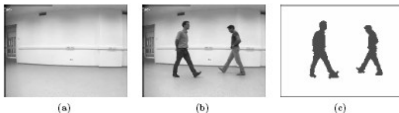
Figure-2: Background subtraction based object detection where (a) is the background, (b) is the current image and (c) is the detected objects [7]
