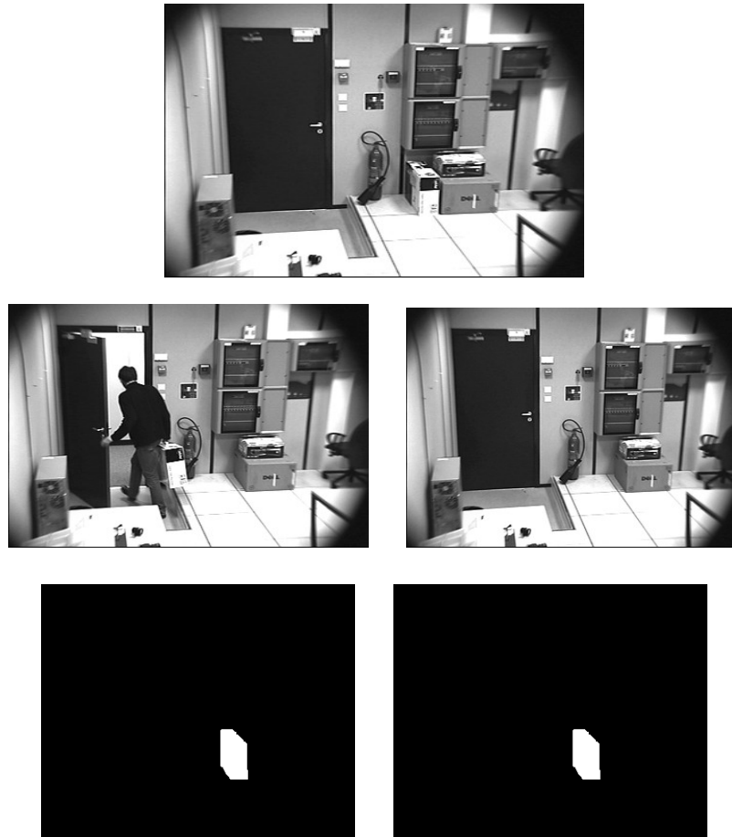
Figure-53: Background, frame samples and foreground object masks of stolen object dataset
