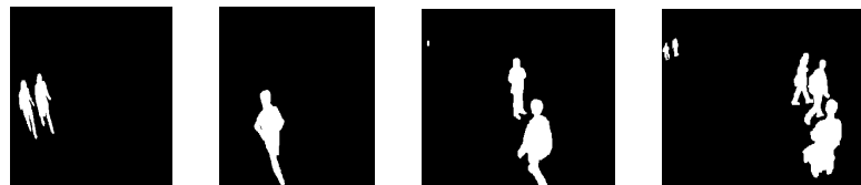
Figure-24: Frame foreground mask samples of a video-surveillance system
