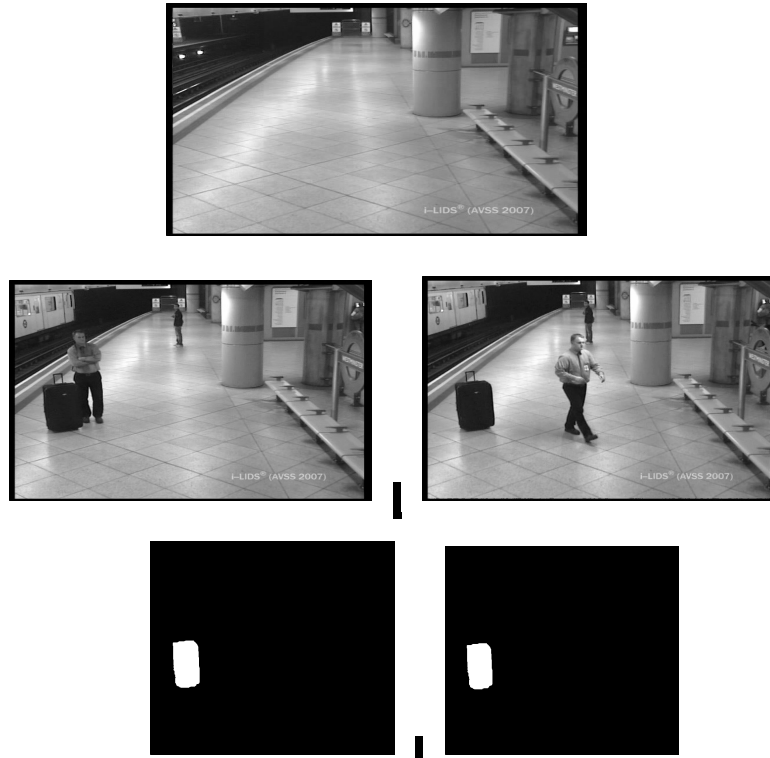
Figure-25: Background, two frames and two object masks of the abandoned object dataset
