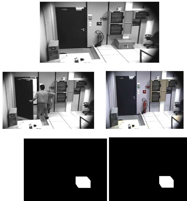
Figure-26: Background, two frames and two object masks of the stolen object dataset
