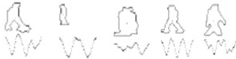
Figure-28: Distance signals graphs for sample human shapes [7]
